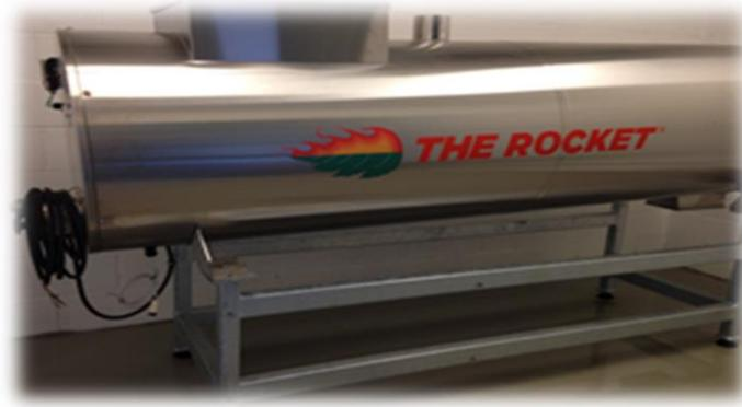
Originally from the United Kingdom, this sophisticated equipment is a hygienic, sustainable system which reduces carbon emissions by eliminating the need for waste disposal transportation. Inside the vessel of the Rocket Composter organic material can transform into high quality compost in only 14 days.
